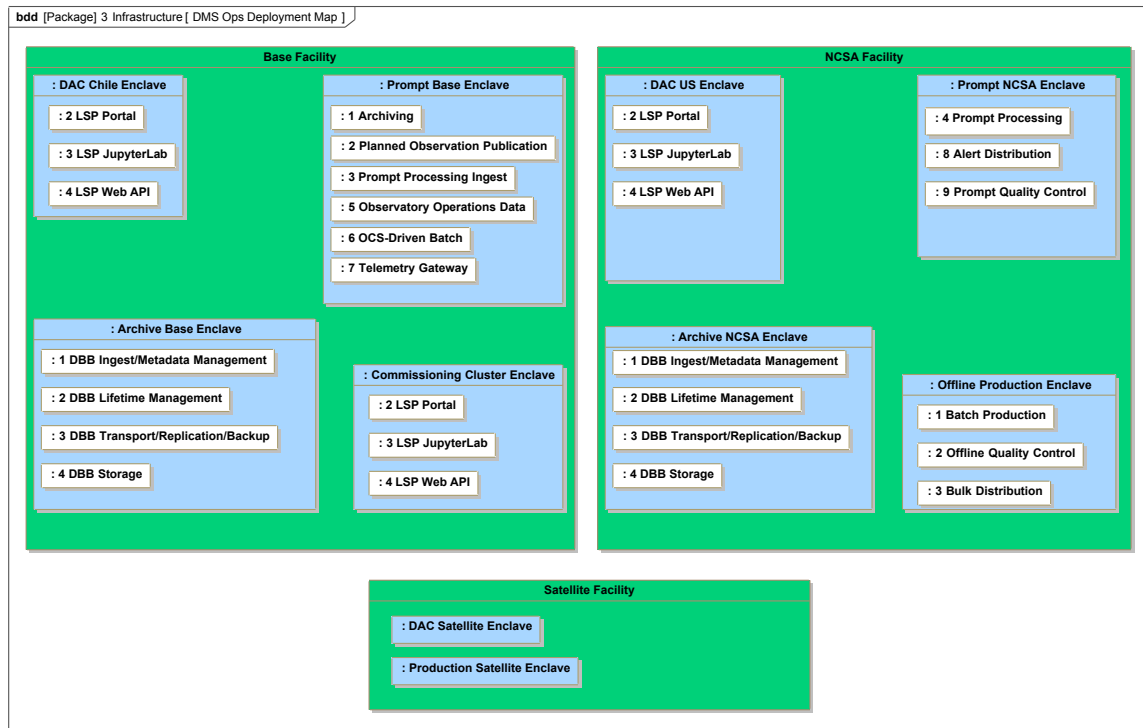
FIGURE 1: DM components as deployed during Operations. Refer to LDM-148 for details of each component.
